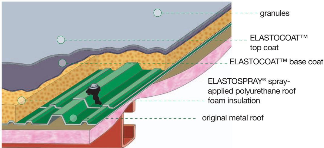
The ELASTOSPRAY® spray-applied polyurethane foam (SPF) roofing system from BASF delivers a cost-effective and sustainable solution for aged and leaking metal roofs – one that economically provides new life to the existing metal roof.
