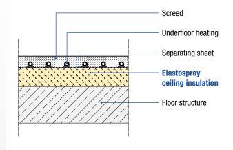
Insulation under the heating screed
