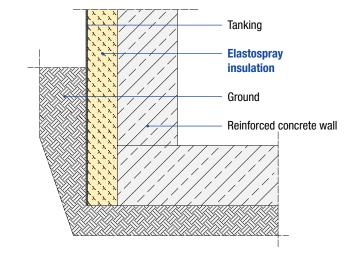
Basement insulation behind tanking
