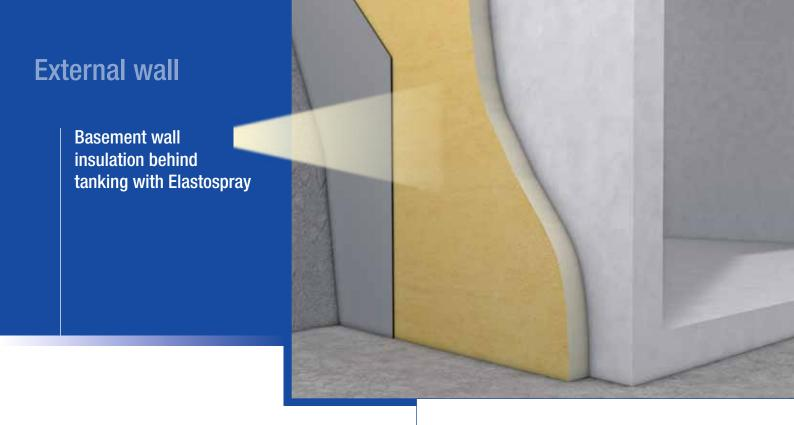
The external walls of buildings usually make up the largest surface area through which heat can escape. Between 100 and 150 kilowatt hours of heating energy escape annually through one square metre of un-insulated wall. This equals approximately 10 to 15 litres of fuel oil or 10 to 15 cubic metres of gas. Basement walls, despite not being visible, are external walls. External thermal insulation (perimeter insulation) of basement walls with Elastospray can reduce energy consumption by up to 90 %.
