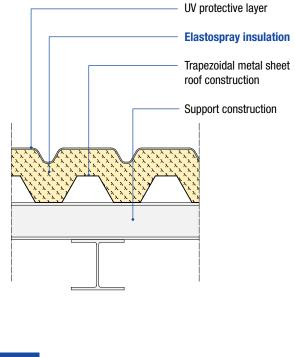
Trapezoidal metal sheet roof with external insulation and UV protective layer
