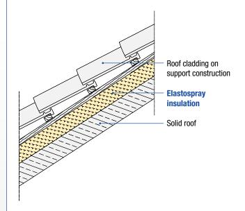
Solid pitched roof with external thermal insulation
