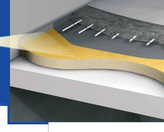
Thermal insulation above the floor slab is advisable where underfloor heating is installed. The insulating layer separates the heated and unheated areas inside a building and in this way reduces any loss of valuable heating energy. Even with rooms only used occasionally, insulation on top of floors with underfloor heating has benefits because the "cold" floor heats up more rapidly and no heat is passed into the floor slab.
