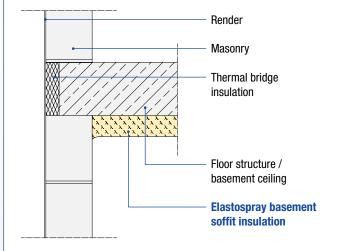
Soffit insulation for unheated basements
